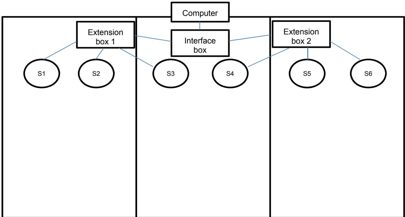
Figure 1. Layout of one of the compartments. 3 sensors are connected to 2 extension boxes, to have 2 sensors in each light treatment.
