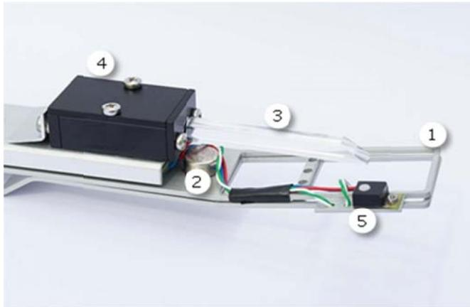
Figure 2. Micro-Moni-PAM: the measuring device or sensor of the Micro-Moni-Set.
