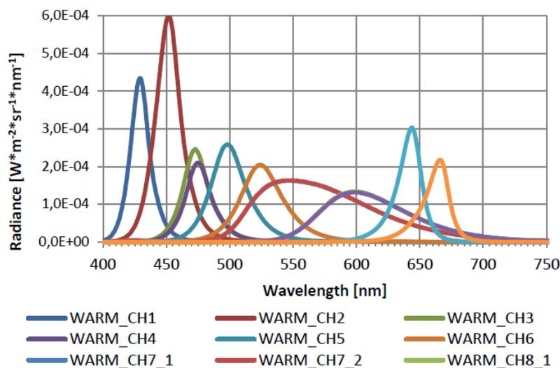
**Figure 1: SPD of the primary channels of the HI-LED 2nd prototype luminaire**
