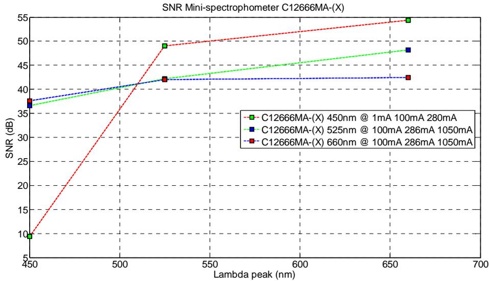
Figure 9. C12666MA-(X) Signal to noise response (SNR)
