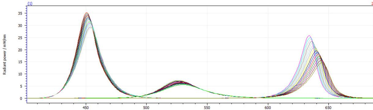
**Figure 1.** Spectral shifts due to the temperature instabilities
