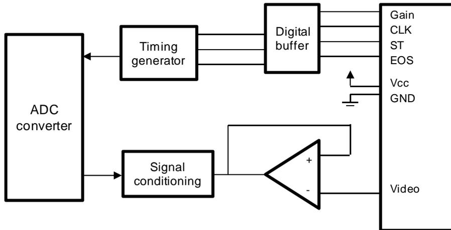
Figure 5. Hardware interface used to communicate with the analog mini-spectrometer module
