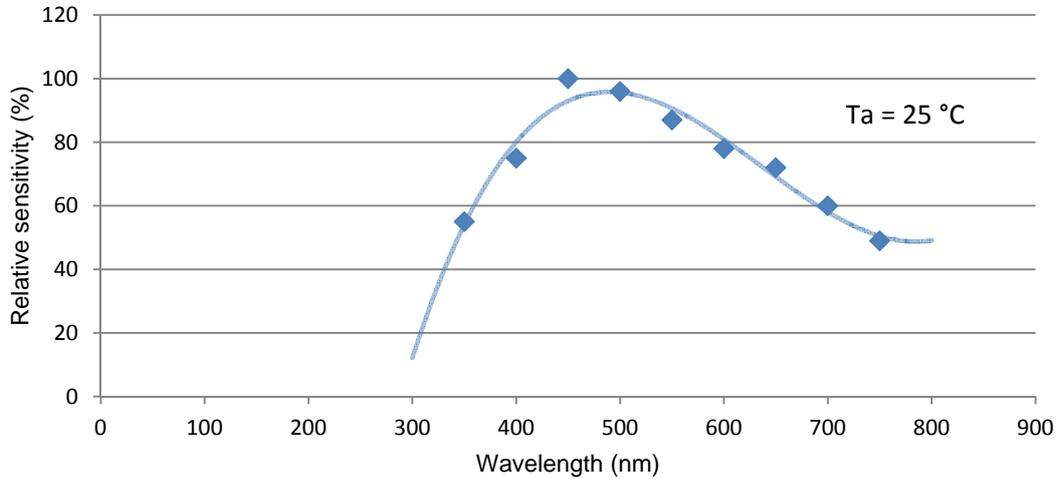
**Figure 3.** C10988MA-01 Relative sensitivity @ Ta= 25°C (340nm - 780nm)
