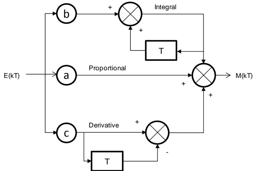
Figure 11. PID controller parallel implementation
