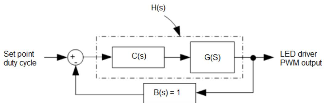
Figure 13. Block diagram of the implemented LED driver controller.
