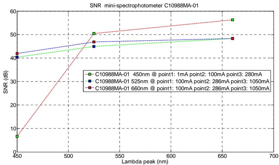
Figure 10. C10988MA-01 Signal to noise response (SNR)
