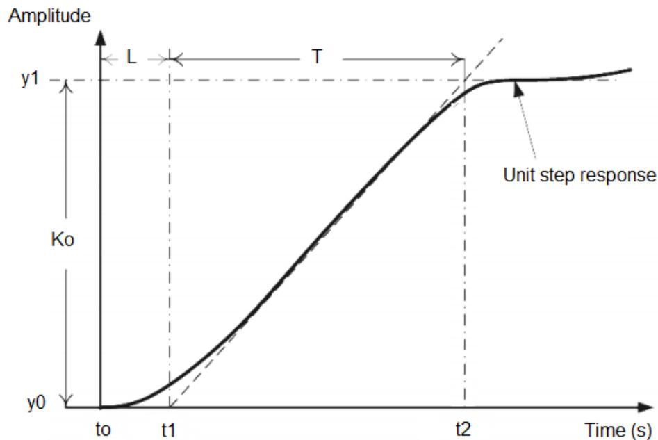
**Figure 12.** Parameters of interest in Ziegler Nichols open loop tuning
