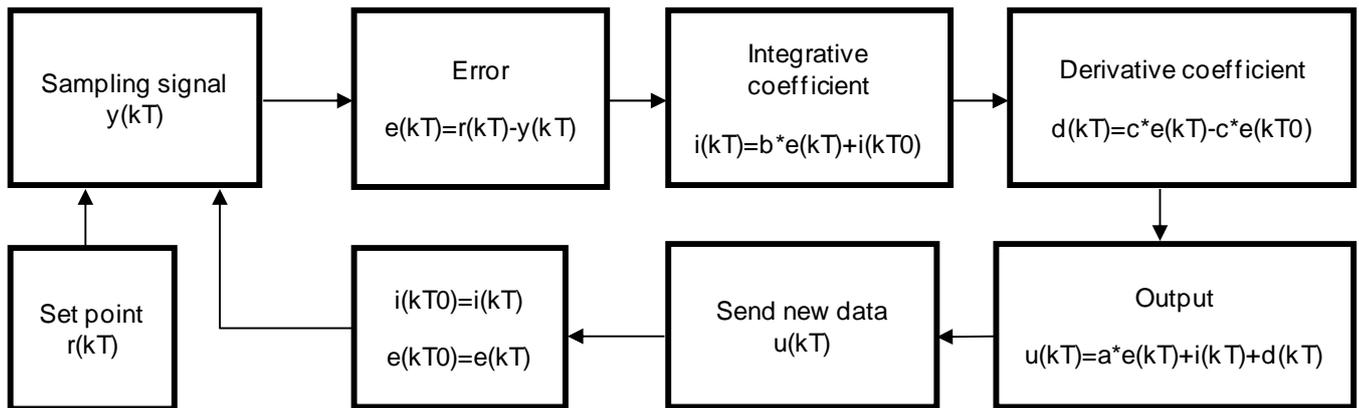
Figure 13. Algorithm used to implement the PID controller in each LED channel
