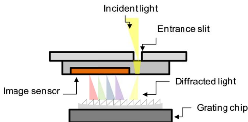
Figure 2. Mini-spectrophotometer architecture
