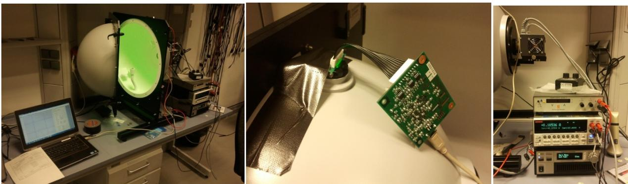
Figure 8. (a) General overview of the setup. (b) minispectrometer attached to a secondary port of the sphere. (c) current sources and measurement equipment
