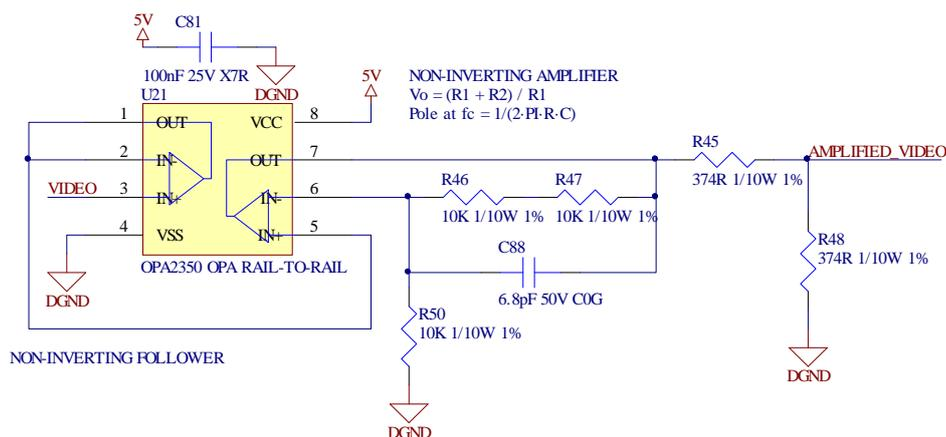
Figure 6. Signal conditioning amplifier module
