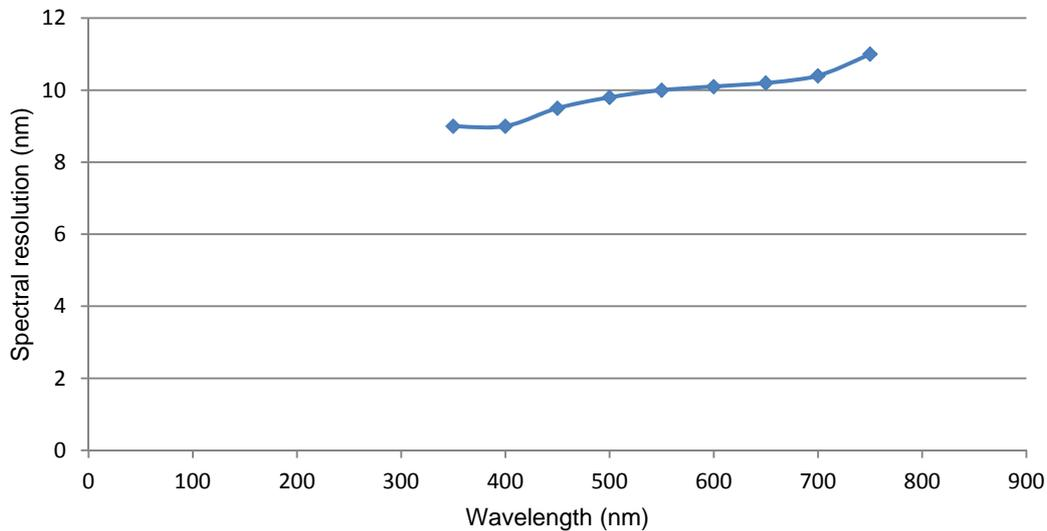
**Figure 4.** C10988MA-01 Spectral resolution @ Ta= 25°C (340nm - 780nm)
